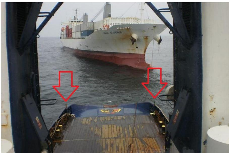
**Figure 4.3.2.2/3:** Photo from a towage conducted by CHRISTOS XXII using a steel wire tow line, where removable poles (indicated by the red arrows) were used. (Image Source: [www.marinetraffic.com](http://www.marinetraffic.com))
