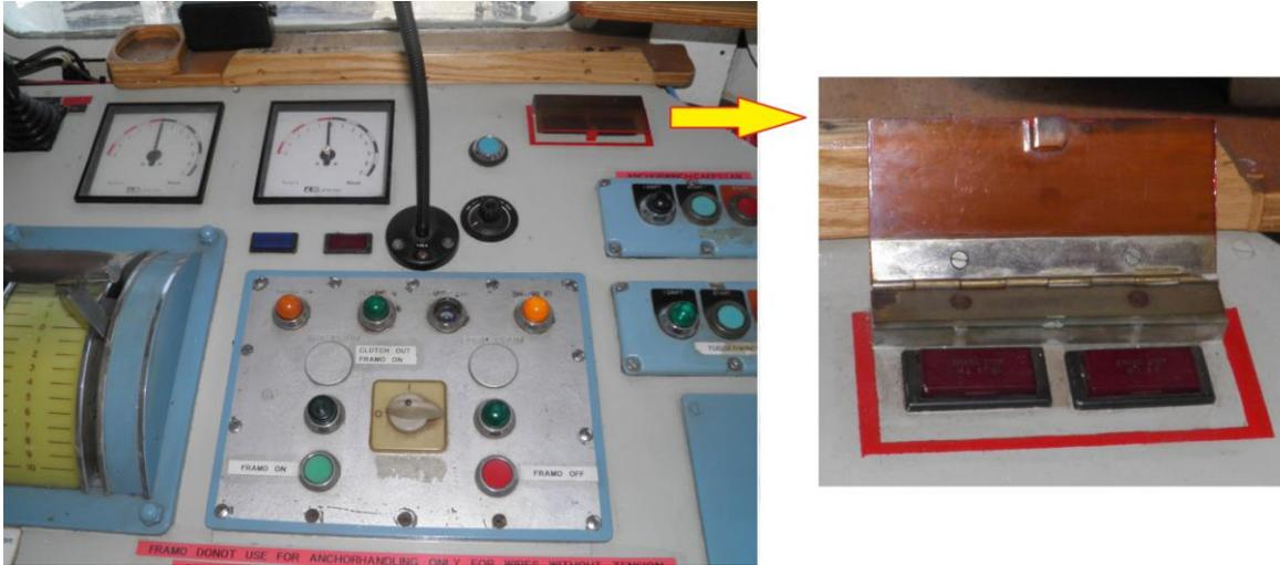
**Figure 3.5/1:** The “EMERGENCY STOP” buttons for both Main Engines, located at the bridge console.
