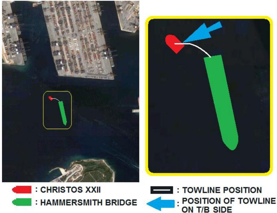
**Figure 3.3/1:** Overview of the vessels' relative position at some point after the towing procedure and prior to the release of the towline by HAMMERSMITH BRIDGE, as estimated by descriptions during the interviews' process.
