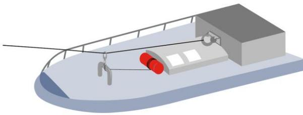
**Figure 4.3.2.3/3:** Gog rope led from a winch, used to vary the length of the gog rope.
